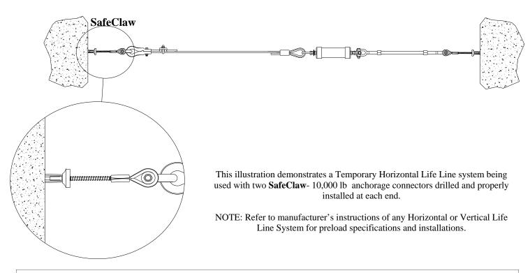
When placing a SafeClaw, Place your thumb inside the anchor loop and your first two fingers around the trigger. Retract the trigger until the spring bottoms out. With your other hand, pinch the two spoons between your thumb and index finger. IMPORTANT; Make sure the cleaning bushing is not wedged between the two spoons. Hold the trigger fully retracted while inserting the unit into bottom of the hole. DO NOT force the unit into the hole. Insert the unit slowly and gently.
