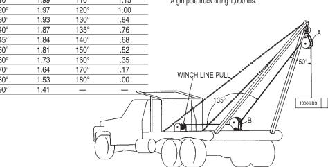
There is no mechanical advantage to a single part load line system, so winch line pull is equal to 1,000 lbs. or the weight being
