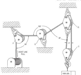
To determine total load on traveling block
