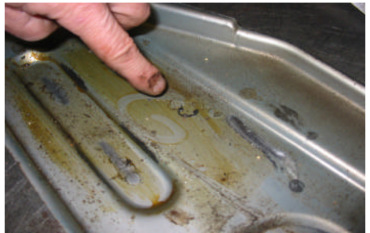
Check for wear or any loose parts (snap rings) inside casing cover.
