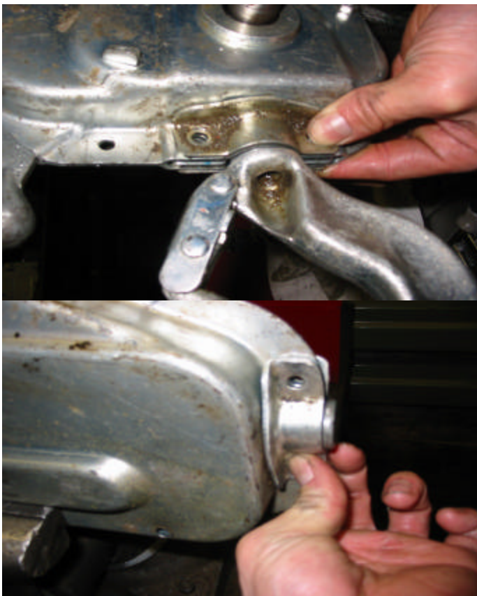
Make sure casing flange is in place for fastening
