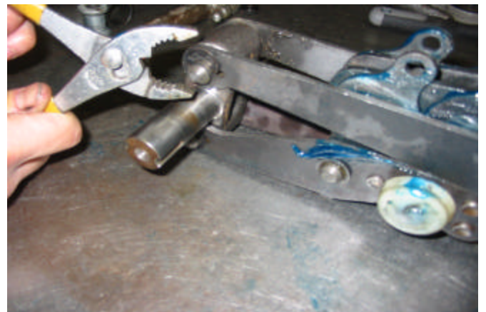
Secure crankshaft connecting pin with pin snap ring.
