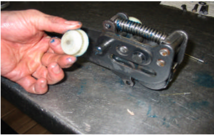
Grease roller and place roller on jaw assembly pin on guide roller. (Position. 034)
