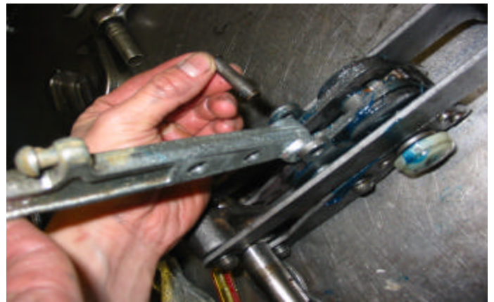
Start reversing lever assembly by fasten lever in place with reversing lever pin (Position. 039)
