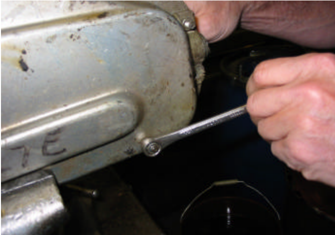
Remove casing screws. 10mm wrench TU-17 / TU-8
