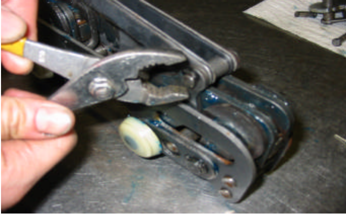
Place spacer and fasten reversing lever connecting rods with reversing lever pin. (Position. 039)
