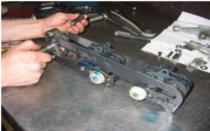
Connect front and rear jaw with crankshaft. (Position. 919)
