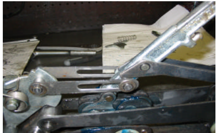
Assemble clutch actuating lever sub assembly to reversing lever. Secure assembly with pin and pin snap ring.
