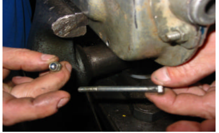
Fasten through casing screw.
