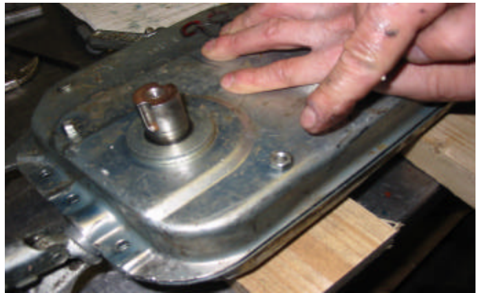
Start tightening all casing screws.
