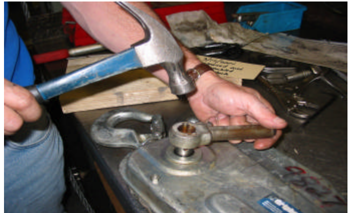
Grease shaft and install power stroke lever on crankshaft. Secure it with 2 new shear pins for TU-17/TU-8 and 3 for TU-28/TU-18. Do not reuse shear pins.
