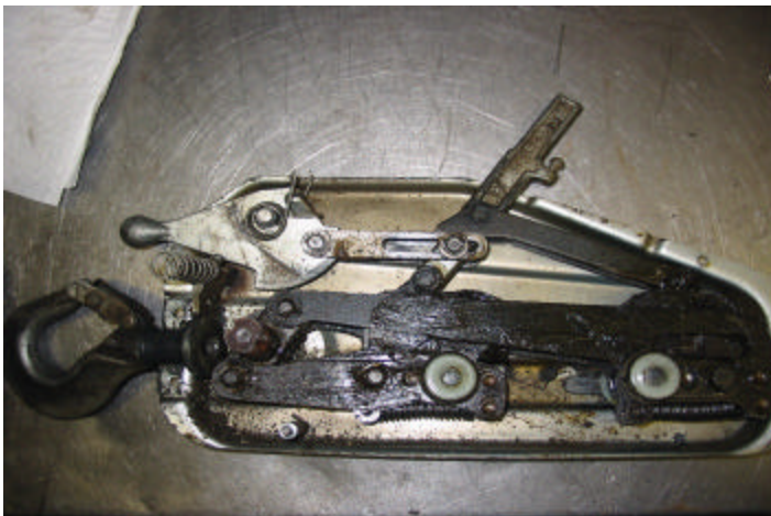
Remove casing cover once casing screws are removed.
