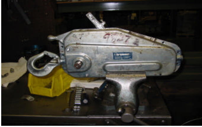
Place hoist on vise for easier assembly.
