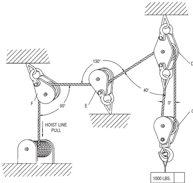
To determine total load on traveling block
