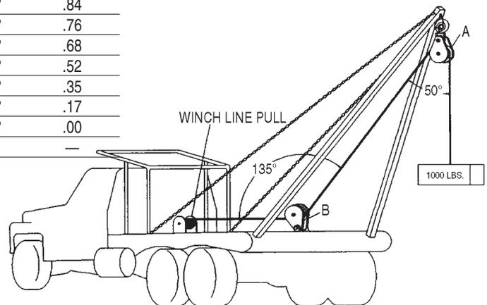
There is no mechanical advantage to a single part load line system, so winch line pull is equal to 1,000 lbs. or the weight being lifted.
