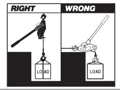
WARNING: These hoists are intended for industrial use and not for lifting or supporting human cargo.
